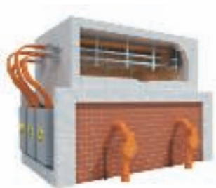
Testing furnace of a materials' testing institute (MPA)
