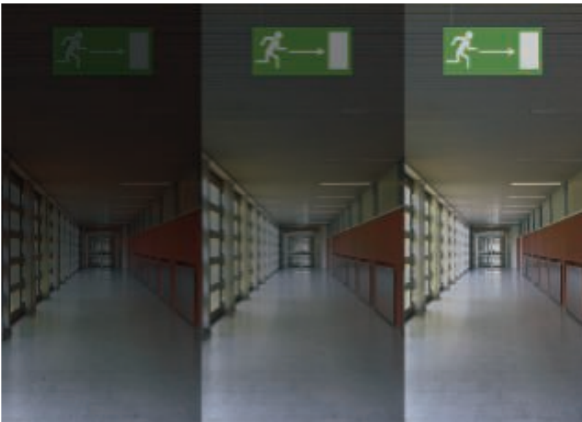
Behaviour of cables in case of fire: PVC-insulated, low-smoke, halogen-free (from left)
